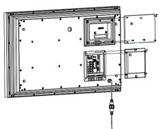
**3** Insert the network board into the monitor, and fix it with the screws.
